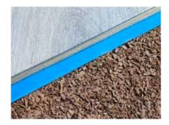
**Defintion:** Floorfixx Balance 020 is a dry levelling fill (according to DIN 18560-2) made of mineral-coated wood chips. Due to the special grain size distribution, Floorfixx Balance 020 is particularly suitable for levelling hollow spaces or height differences that need to be accommodated.
