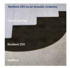
**Defintion:** Resilient 250 is a high performing acoustic resilient layer that has been designed to significantly reduce impact sound. It can be used as used as a soft floor covering or as an acoustic underlayment.
