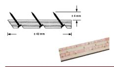
**Defintion:** For bonding to concrete and wood. The additional row of pins deliver better grip combined with an extra wide plywood base for better power distribution. Recommended for long stretch fits of 10m / 30ft or more.
