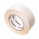
**Defintion:** Tapiton Flex is a high-quality double-sided carpet/vinyl tape for the professional user. Highly plasticizer resistant and therefore suitable for LVT, vinyl and carpet. Due to its polyester carrier, it is very dimensionally stable. Can be processed by hand. Can be processed on any desired subfloor.
