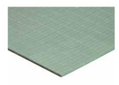
**Defintion:** Duralay LVT Dryback Underlay is a versatile underlay solution which can be used to install 'Dryback' luxury vinyl tiles. Reducing subfloor preparation time. Installation is quick, clean and simple. The underlay is loose laid over the subfloor or existing flooring. The release film is peeled back to expose the adhesive, the new flooring is then positioned and pressed onto the underlay's high grab backing.
