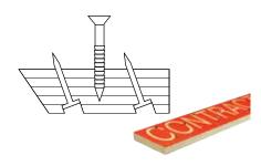
**Defintion:** For particularly heavy stretch installations. It is 42 mm wide and has 3 rows of carpet holding pins. Medium pin height with no floor nails. Allows the fitter to install by nailing or adhering the gripper to the floor, depending on the installation.
